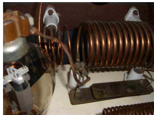
Figure Dec05—Photo 6. End turn of main inductor shorted with solder.
