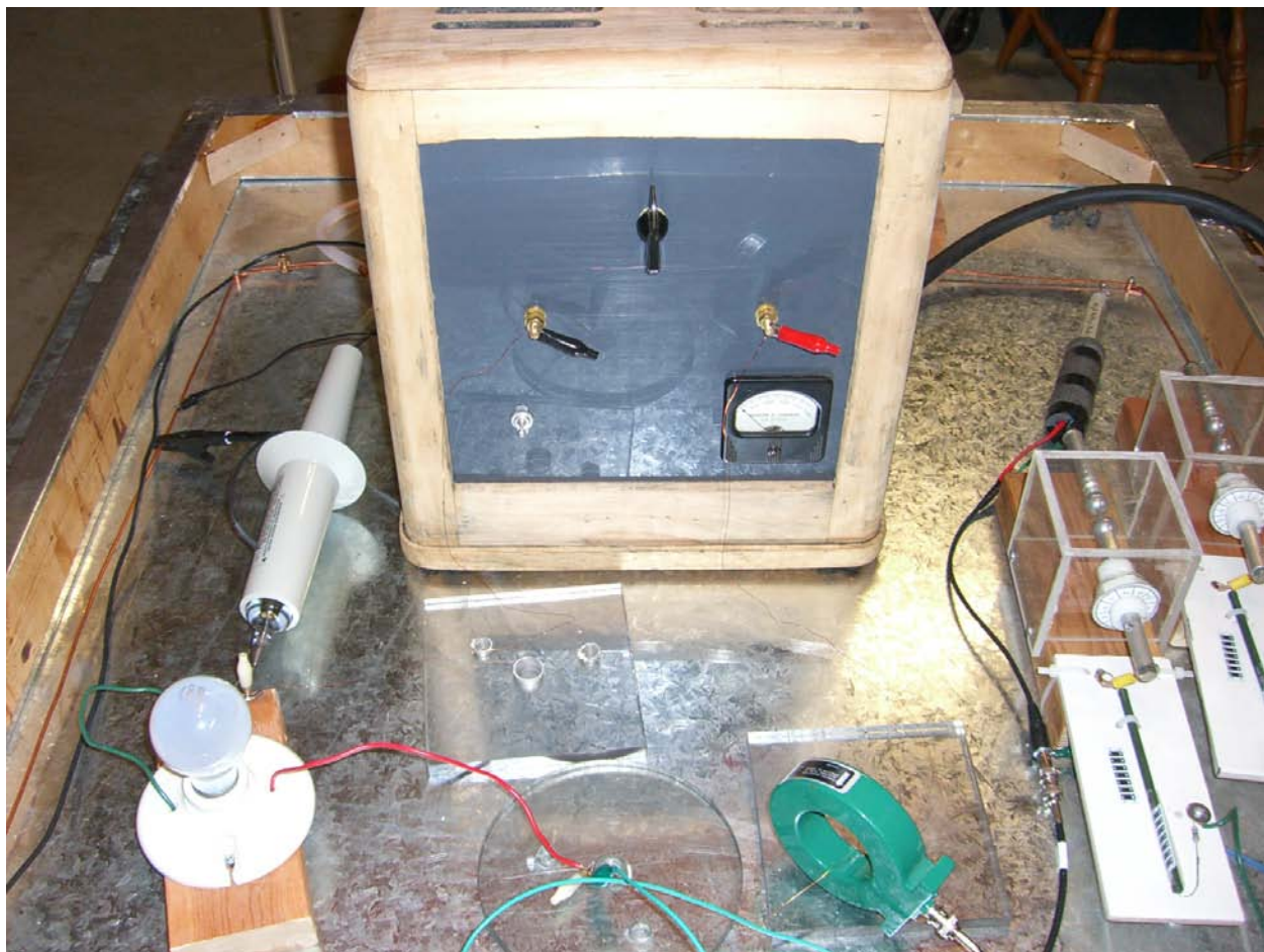
Figure Dec05 – Photo 13. General Lab Setup with 30-gauge wire from HF terminals to lamp wires.
